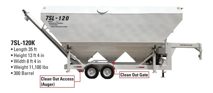
**Mobile and Durable** 6 Inch Auger 700 lbs/min 8 Inch Auger 1500 lbs/min **Towed with 1 Ton Pickup Optional Load Cells Optional Auto Control Clean Out Gate**
